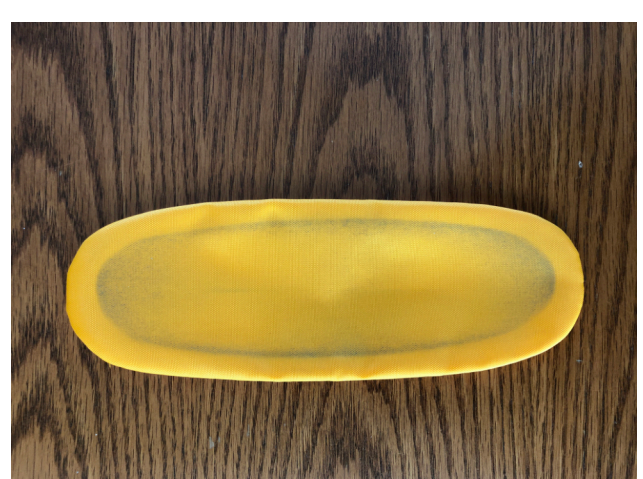
Figure 18 - Used brush pad showing greater wear around the edges
