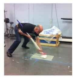
the ice, as well as the number of brush strokes per second. We captured the detailed force and motion components involved in brushing using an AMTI BP400600-100 force plate, located in the Kinesiology Laboratory at the School of Human Health and Performance at Dalhousie
