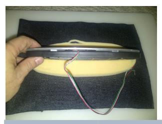
instrumented aluminum plate was placed in a custom-made brush pad to act as a bending load cell and measure the vertical contact force between the brush pad and the ice. The data is streamed wirelessly, in real time, to a laptop close by and operated by the coach. The broom measures and transmits the force readings at a rate of 100 readings per second such that each full stroke (a combination of the push portion and the pull portion) will have
