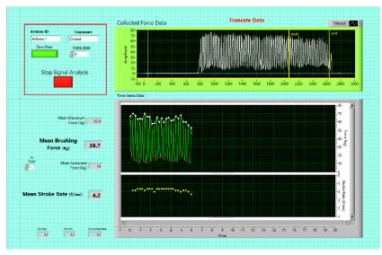
Once the yellow selection bars have been used to identify the relevant data range, the software isolates the data set (shown in the Time Series Data window) and conducts a peak detection process to identify maximum force (white line/dots) and sustained force (red line/dots) values for each individual stroke. In addition, the timing of each stroke is
